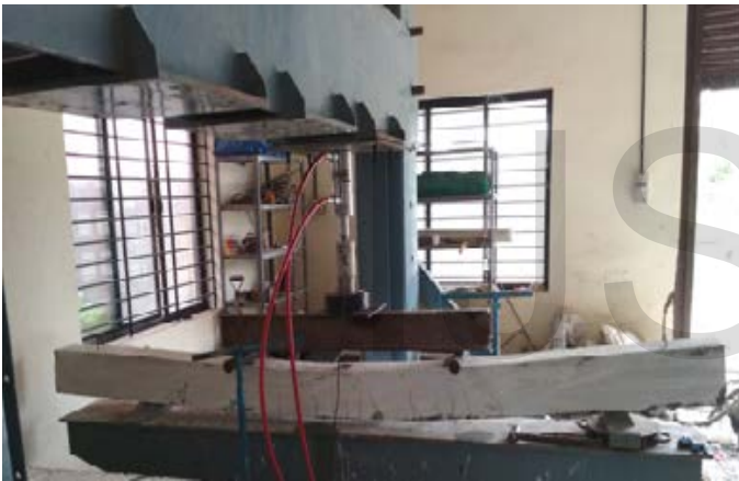
Fig.9 Beam after loading
