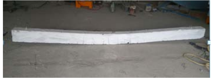
Fig.11 Ductile behavior of rice husk ash beam
